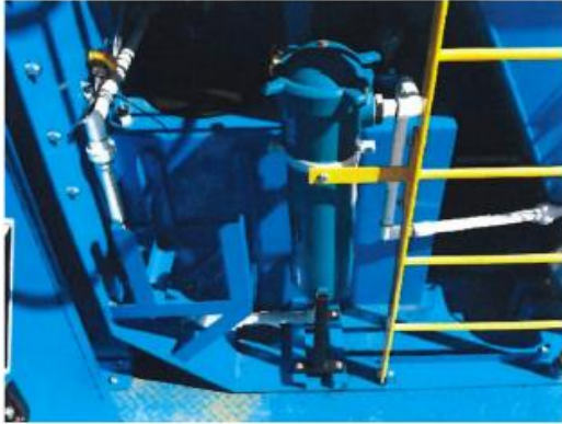
Filter Housing Assembly carries a 50 micron filter bag that is easily changed out when necessary
